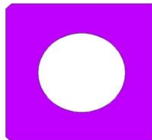
Hollow Cored Square Section Pile
